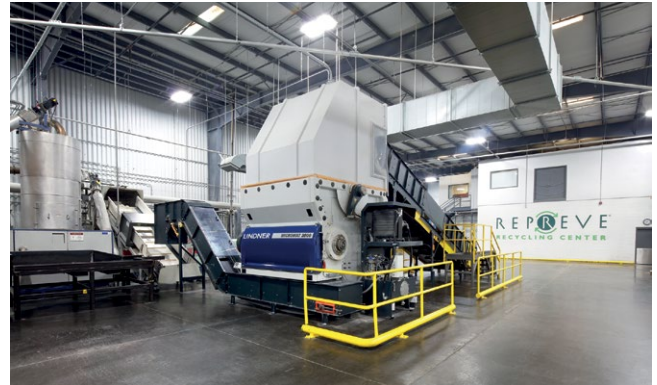
At Unifi, Inc. three Lindner Micromat 2000 work 24/7/365 to prepare plastics and textile waste for its journey to extrusion, spinning and finally winding the fibers (Images Copyright: Lindner Recyclingtech)
