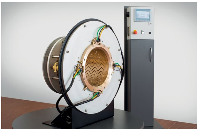
The motor-controlled calibration sleeve for controlling the diameter and the ovality of the pipe (inline). Designed for plastic pipes from 280 up to 2400 mm (also available in inch sizes)
