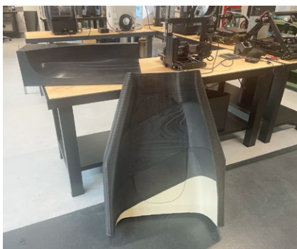
3D-printed laminating molds made with LUVOCOM 3F
